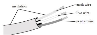
(a) (i) Draw one line to link the name of each part of the cable to its description.
